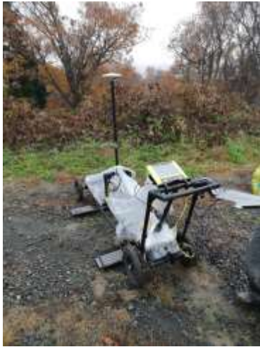
Fig 3 GPR unit mounted with the GNSS.
