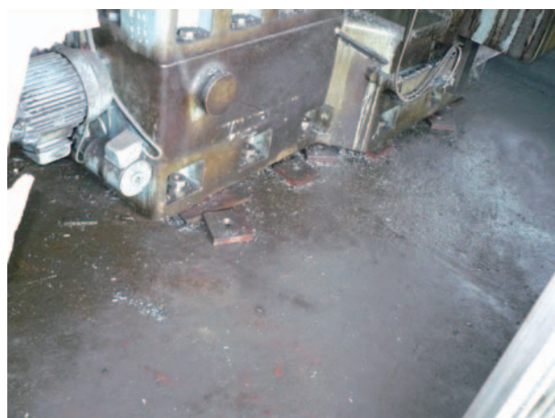
Fig. 2 A milling machine weighing approx. 10t that fell off leveling blocks.
