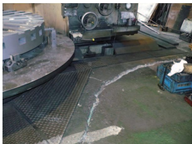
Fig. 3 A large size vertical lathe and cracked floor around it. Installation with anchor bolts made the machine be fixed securely.
